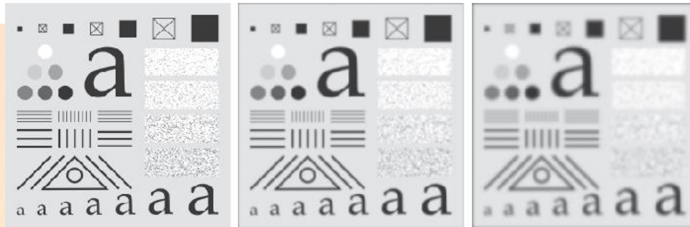
FIGURE 3.36 (a) A test pattern of size 1024 \times 1024 . (b) Result of lowpass filtering the pattern with a Gaussian kernel of size 21 \times 21 , with standard deviations \sigma = 3.5 . (c) Result of using a kernel of size 43 \times 43 , with \sigma = 7 . This result is comparable to Fig. 3.33(d). We used K = 1 in all cases.
