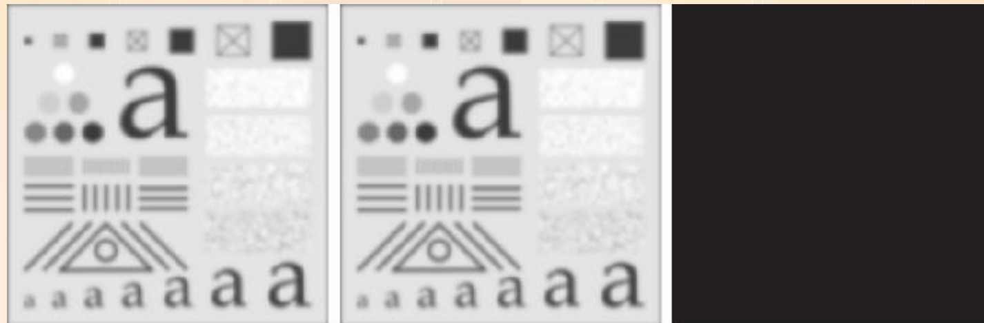
FIGURE 3.37 (a) Result of filtering Fig. 3.36(a) using a Gaussian kernels of size 43 \times 43 , with \sigma = 7 . (b) Result of using a kernel of 85 \times 85 , with the same value of \sigma . (c) Difference image.
